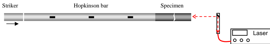
Fig.1 Principle of a modified experimental arrangement used for estimation of dynamic strength in tension
