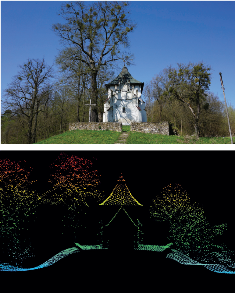
Figure 1. The Greek Catholic church (14th century) in Posada Rybotycka lying within the scanned area. The oldest existing Eastern rite church in Poland: top – a regular digital photograph, bottom – a 10 m deep profile of the obtained point cloud. Points coloured by elevation
