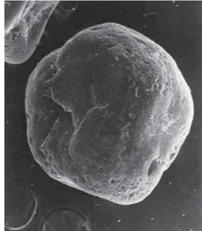
Figure 18. Spheroidal, rounded and matted grain of quartz with low and partially high relict relief of large conchoidals with rounded edges, convex edges covered with granular breakages and splittings of mechanical aeolian tooling (magnification 72x, Ees horizon, depth 15–20cm, uppermost part of the coastal berm, Hel Peninsula).
