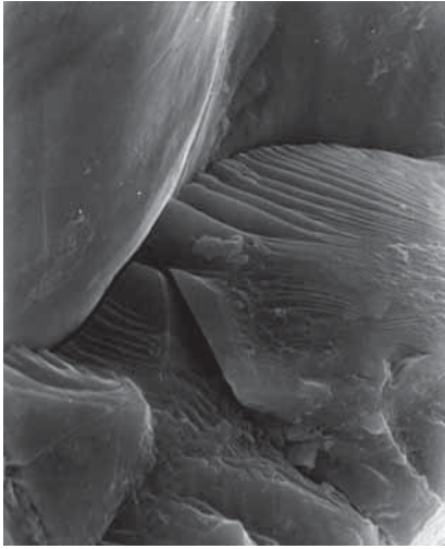
Figure 21. Walls of multidirectional imbricate conchoidals with crevices due to large-block frost chopping by the edge of the angular grain that has been subject to powerful mechanical weathering (magnification 3000x, BvtBfe horizon, depth 10–14 cm, Kevo).
