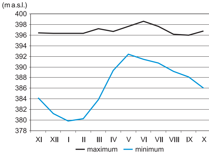
Figure 7. Extreme water levels in the Klimkówka Reservoir in the annual cycle, for the years 1996-2011.
