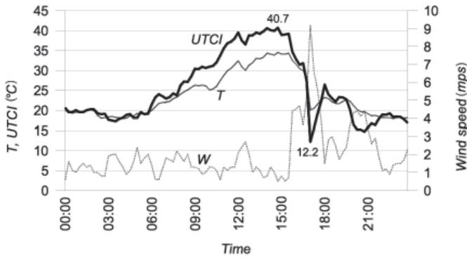
Figure 7. The course of the UTCI, air temperature ( $T$ ) and wind speed ( $W$ ) during the hottest day of 2009 at the Praha-Libuš station (July 23).
