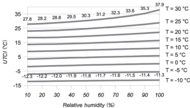
Figure 5. The dependency of the *UTCI* on relative humidity ( $T_{mrt}=T$ ,  $W=1$  m·s<sup>-1</sup>).
