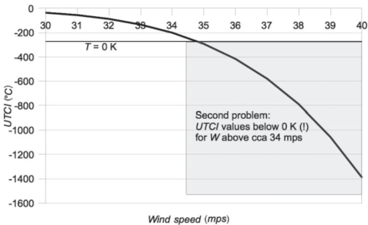
Figure 11. The problem with the *UTCI* for wind speed above 30 m·s<sup>-1</sup>.
