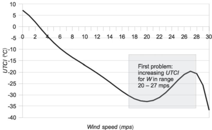
Figure 10. The problem with the *UTCI* for wind speed above 20 m·s<sup>-1</sup>.
