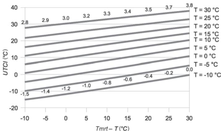
**Figure 3.** The dependency of the *UTCI* on the difference between mean radiant temperature and air temperature  $T_{mrt}-T$  (for  $W=1\text{ m}\cdot\text{s}^{-1}$ ,  $H=50\%$ ).
