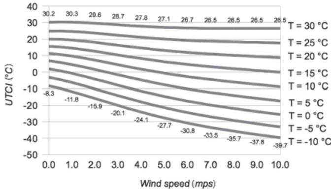
Figure 4. The dependency of the *UTCI* on wind speed ( $T_{mrt}=T$ ,  $H=50\%$ ).
