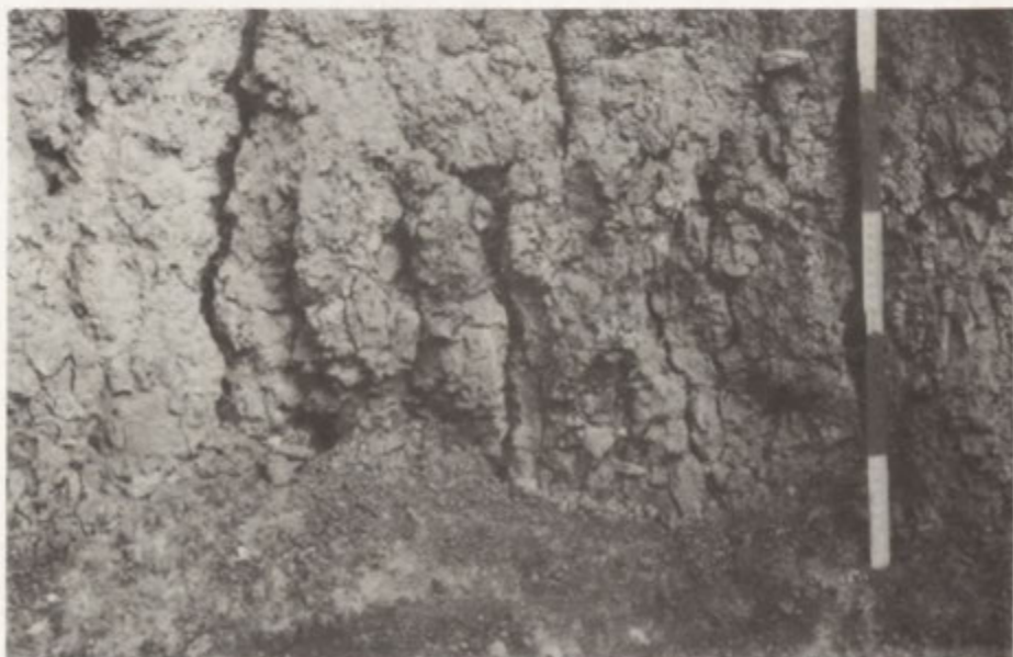
Photo 7. Talus cone composed of fragments of cohesive deposit (Pleistocene varved clay). Bełchatów Browncoal Mine, May 1991
