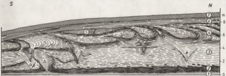
Fig. 9. Loess structure in brickyard at Łopatki, Lublin Upland 1 – red loess, 2 – fossil soil, 3 – grey-yellow loess, 4 – solifluction loess, 5 – sand, 6 – loess deluvia, 7 – soil, a–e – ice wedge casts
