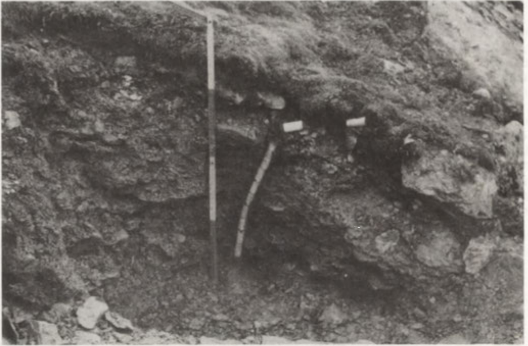
Photo 2. Displacement of wooden pegs in five-year period (1979–1984) on Jens Erikfjellet slope (Hornsund region). Concave down-slope curve of movement involved the entire active layer. Photo H. Chmal
