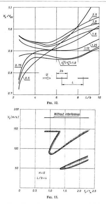
By contrast with the biplane configuration, which has a characteristic feature of monotonic decrease in the critical flutter speed with decreasing distance between the airfoils, there is no such feature for profiles arranged one behind the other. The influence of the aerodynamic interference may be different for different configurations of airfoils, depending
