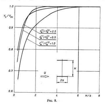
the axis of ordinates taking into account the interference. Each particular curve corresponds to a different value of the ratio of frequencies of torsional vibration, for  $f_h^{(1)}/f_h^{(2)} = 1.4$ . The influence of the aerodynamic interference in airfoil configurations of various ratios of flexural rigidities is analogous (Fig. 9).
