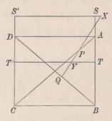
say AB, CD are directrices, and BC, AD are generatrices, the two reciprocal lines being the diagonals AC and BD of the skew quadrilateral. Taking on AC a point P and on BD a point Q, the theorem is that, if PQ meets the surface in the points
