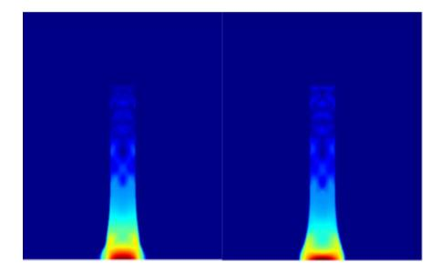
Figure 1: Comparison of the von Mises equivalent stress  $\sigma_v$  in a Taylor Anvil test. On the left the result with the reference map technique and on the right without the reference map. Observe the numerical diffusion near the bottom in the non-reference map result.
