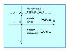
Fig.1. Lossless (elastic) Love wave waveguide (surface layer plus substrate) loaded at the surface  $x_2 = -D$  with a lossy viscoelastic medium of the shear modulus G and viscosity n.
