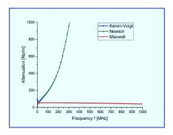
Fig.2. Attenuation of the Love surface wave, propagating in a lossless elastic waveguide, loaded with 3 different types of lossy viscoelastic materials, i.e., Kelvin-Voigt, Newton and Maxwell. Low, medium and high frequency limits:  $tan\delta \in [0.127 - 127]$ ,  $G = 5 \cdot 10^4 Pa$ ,  $\eta = 1 mPas$ .
