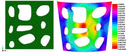
Figure 1: (a) Scan of the original 3D trabecular bone sample, (b) 2D section, and c) Distribution of equivalent strain due to in-plane bending.
