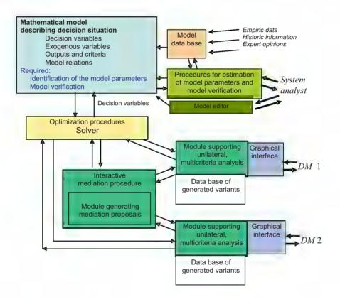
Figure 2: General scheme of the computer-based system.
