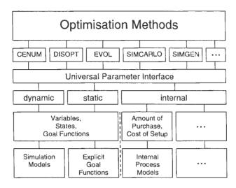
Figure 3. The ISSOP optimisation architecture
