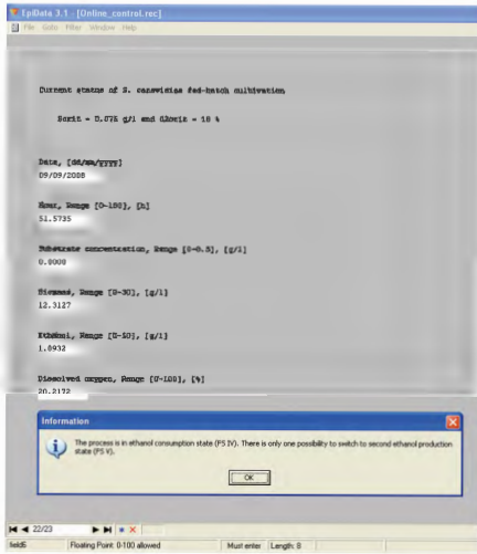
Figure 5: Advisory system and a part of GN model at ethanol consumption state (FS IV)
