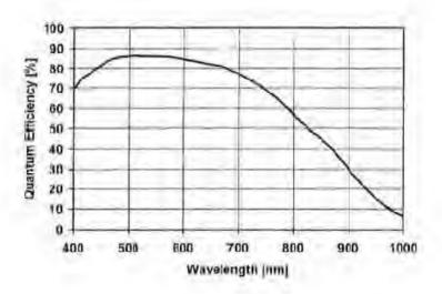
Fig. 5. Typical QE for back-illuminated backside-thinned CCDs. This figure comes from [7].
