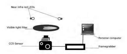
Fig. 2. Device schematics.
