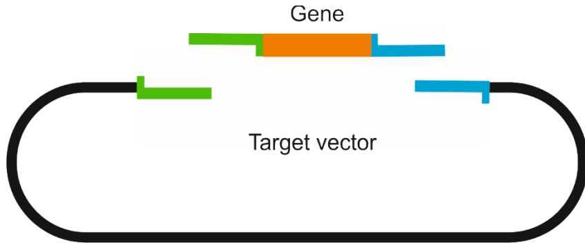
Figure 9. The picture presents an insert and a vector with complementary overhangs after treatment with T4 polymerase
