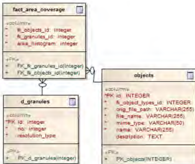
Figure 7: Schema of ROLAP cube that stores granules histograms used to calculate coverage
