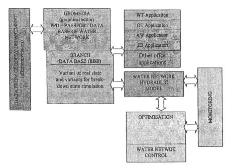
During testing the tool programs connected with numerical map and enabling the cooperation among the numerical map, the hydraulic model and the monitoring system, it appeared that the additional program modules performing managing functions and some other functions, would be useful. There are the following additional preferable modules (applications):
