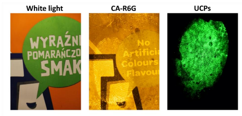
Figure 3.53 5-day-old fingerprint deposited on a Fanta can developed with either CA-R6G or \beta -NaYF 4 :Yb,Er-2-SiO 2 -Ph particles and imaged under 530 nm or 980 nm light excitation, respectively
