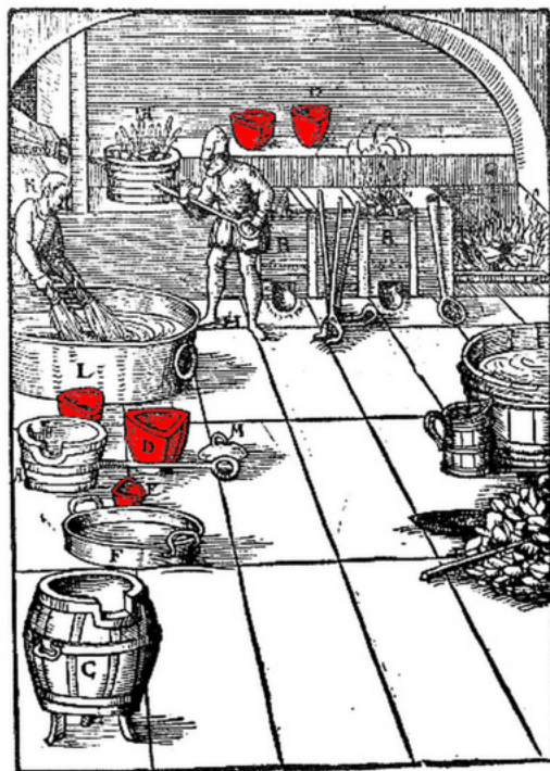
Fig. 3. Presenting the process of assaying the silver content (after: Ercker 1974: 49).
