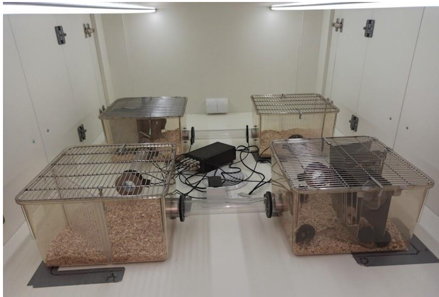
Figure 3. Eco-HAB system inside, soundproof designer rack floor. Each level contains autonomous, individually-lit and -ventilated Eco-HAB, enabling simultaneous, high-throughput experimentation.
