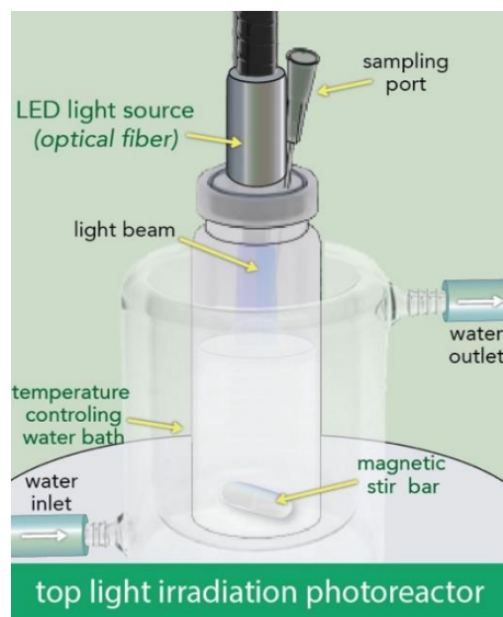
Scheme 3.1. Schematic illustration for the utilized setup for the photocatalytic studies. (Represented from the open access article [123])
