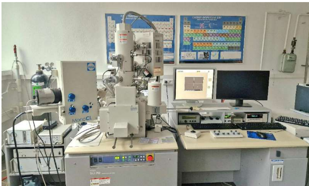
Figure 4.2. Hitachi SU70 scanning electron microscope equipped with an additional Gatan MonoCL cathodoluminescence attachment, the Institute of Physics, IPPAS.
