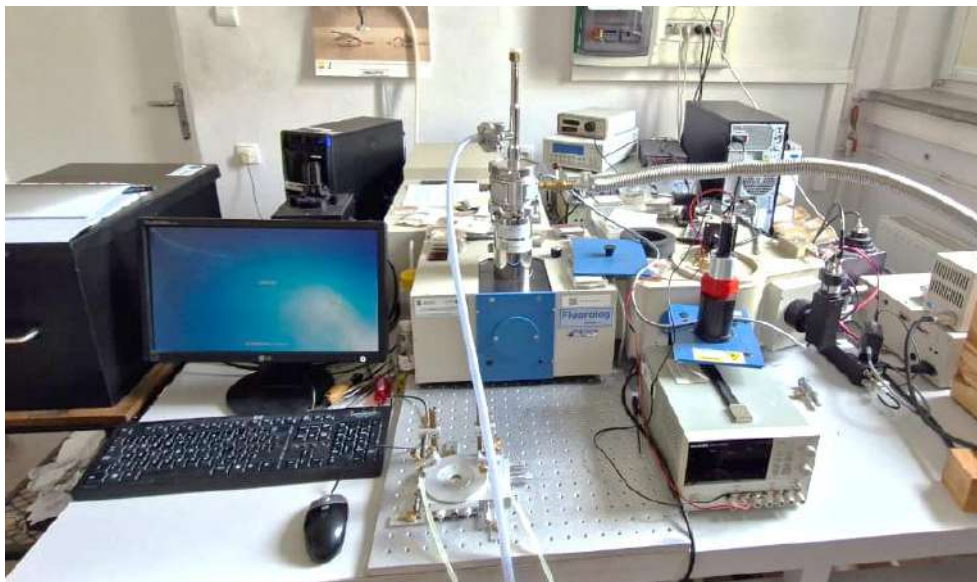
Figure 4.4. A Horiba Fluorolog-3 spectrofluorometer coupled to a cryostat is used for both room temperature and low-temperature photoluminescence measurements at ambient pressure; the Institute of Physics, IPPAS.
