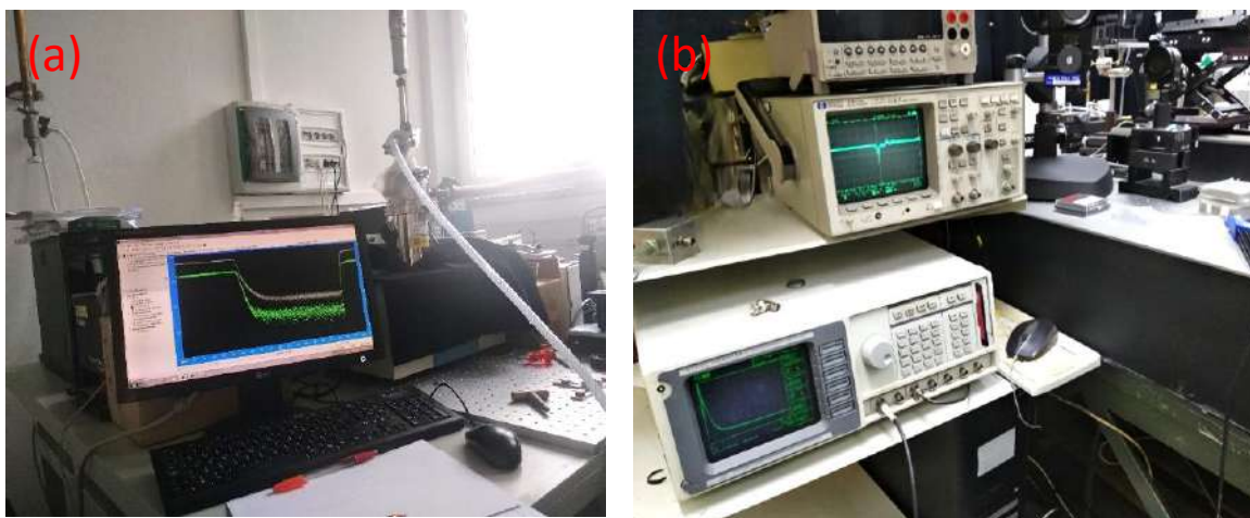
Figure 4.6. Luminescence decay measurements at (a) room temperature or low temperature, and (b) high pressure, the Institute of Physics, IPPAS.
