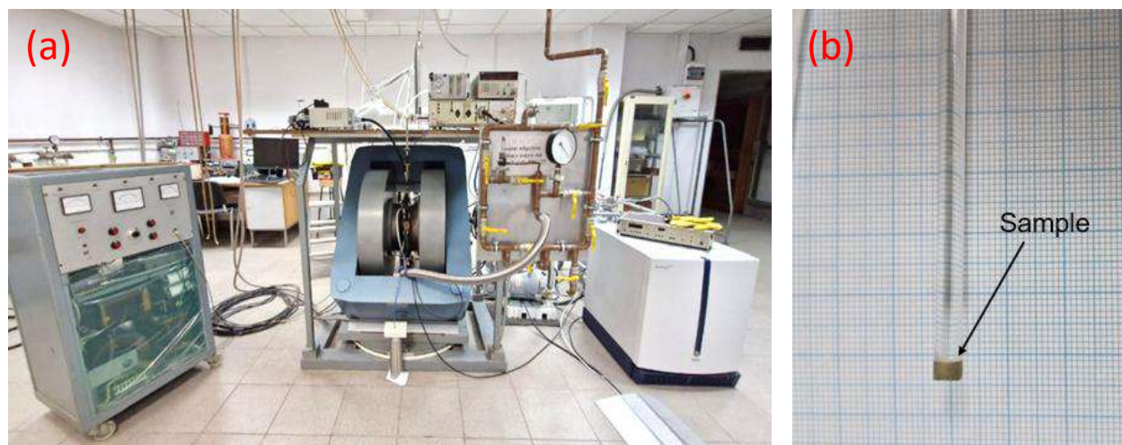
Figure 4.12. (a) Bruker EMX EPR spectrometer used for the study, (b) an iron ( \text{Fe}^{3+} ) doped \text{LiGaO}_2 single crystal sample attached to a quartz tube for EPR measurement, the Institute of Physics, IP PAS.
