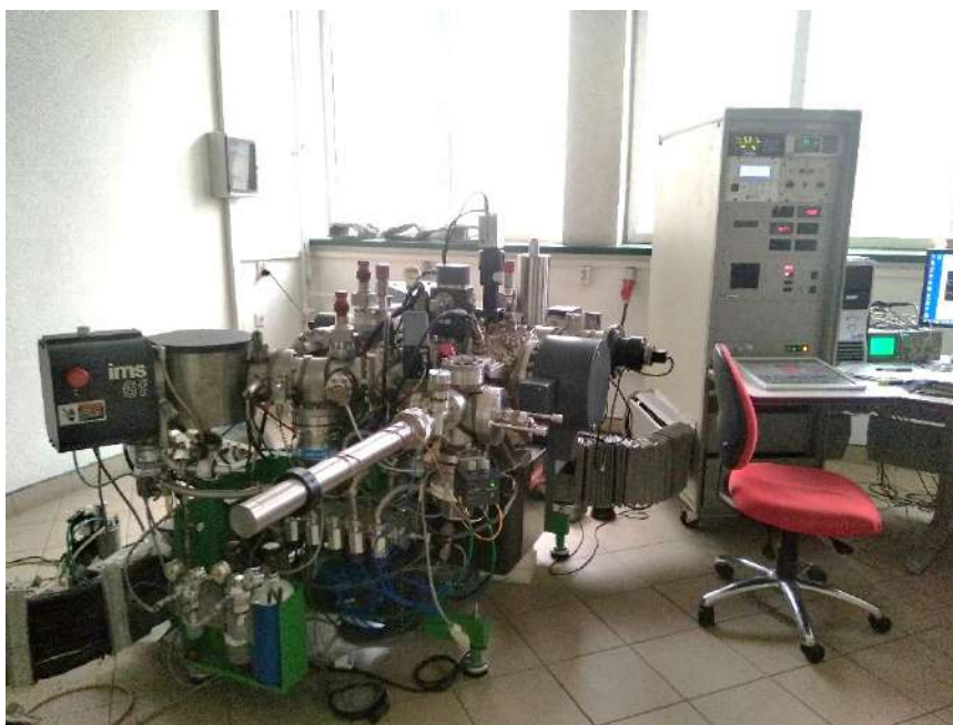
Figure 4.13. The CAMECA IMS6F spectrometer used for the SIMS study, the Institute of Physics, IPPAS.
