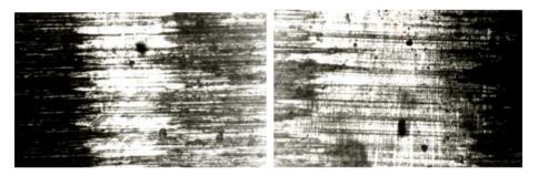
a. Fresh lubricant b. Used lubricant Figure 2. Wear trace for LHP 46 oil
