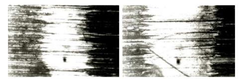
a. Fresh lubricant b. Used lubricant Figure 1. Wear trace for 15W40 oil
