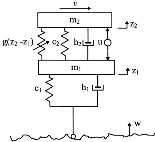
FIGURE 3. Model of nonlinear suspension system (Eq. (24)).
