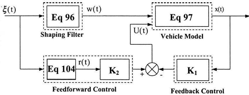
FIGURE 12. Block diagram representation of feedforward and feedback terms of active control in linear model with preview information [52].
