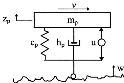
FIGURE 6. Active suspension model (Eq. (78)).
