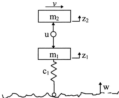
FIGURE 1. Model of suspension system (Eq. (1)).
