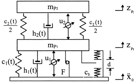
FIGURE 8. Adaptive active suspension model (Eq. (86)).
