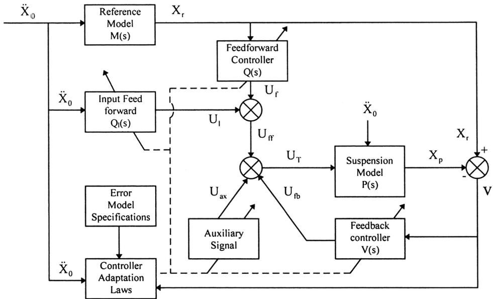
FIGURE 10. Block diagram representation of adaptive active control system [9].
