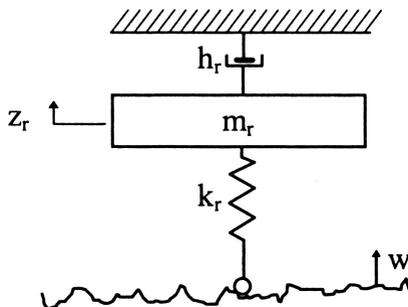
FIGURE 7. Sky-hook damping reference model (Eq. (81)).
