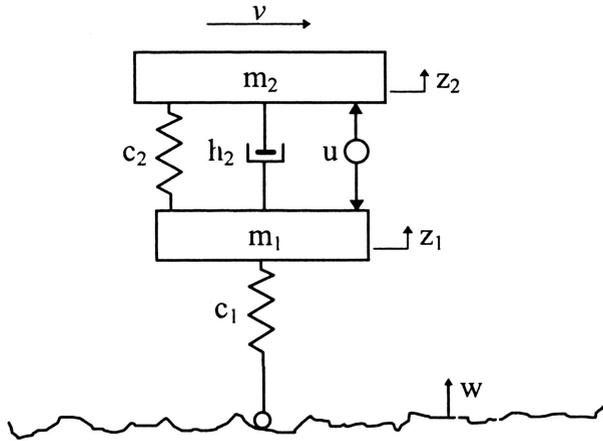
FIGURE 2. Model of linear suspension system (Eq. (18)).
