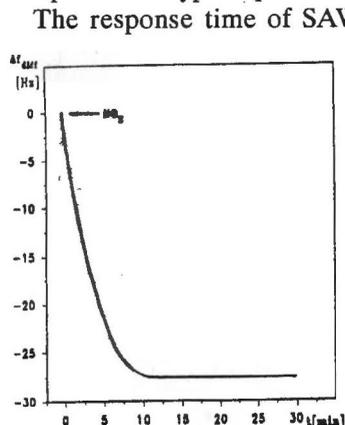
Fig. 8. The differential frequency change versus time for  $\alpha$ -PcCu covered SAW device on lithium niobate (coating mass -  $5 \times 10^{-7}$  g).
