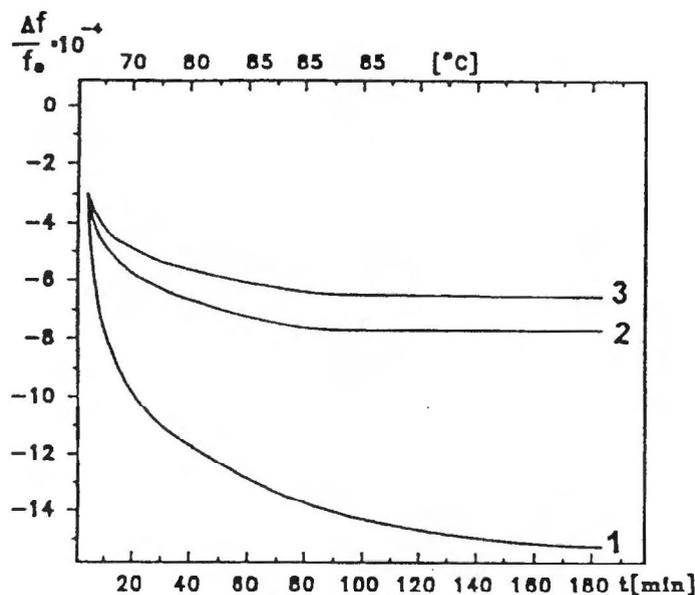
Fig. 6. The relative frequency shift of PcCu-coated delay line on quartz substrate during heating up to 85°C.
