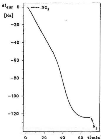
Fig. 9. The differential frequency change versus time for  $\beta$ -PcCu SAW device on lithium niobate (coating mass -  $5 \times 10^{-7}$  g).
