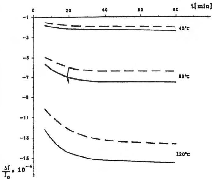
Fig. 5. The relative frequency shift of PcCu-coated and uncoated delay lines on quartz substrate during heating up to three different temperatures:
