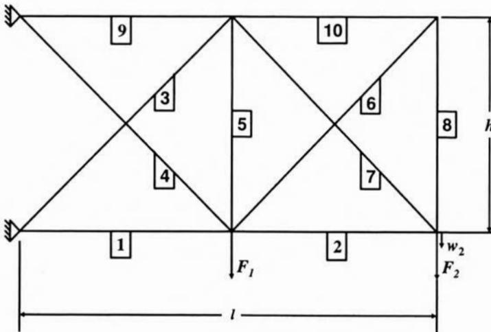
FIGURE 1. Statically system of the ten bar truss.
