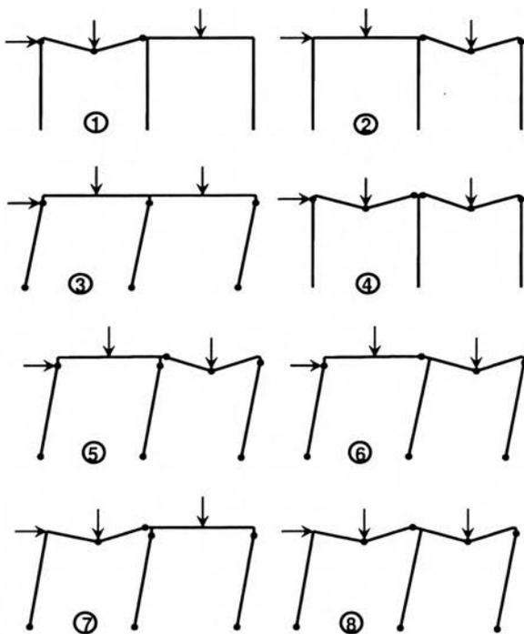
FIGURE 4. Failure modes of the frame.
