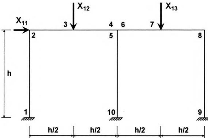
FIGURE 3. Loads and statical system of the frame.
