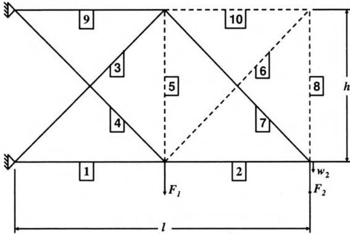
FIGURE 2. Optimized ten bar bar truss (dashed bars are zero bars).
