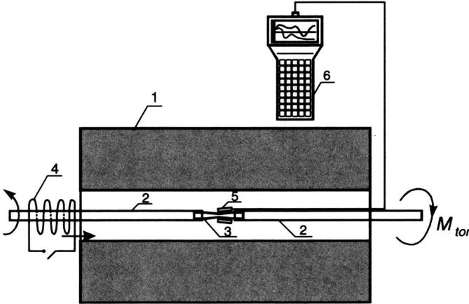
FIGURE 2. The scheme of the experimental set-up for gauging magnetic field on a surface of demagnetized ferromagnetic sample under condition of the absence of the internal field  $H_i$  and external field  $H_e$ : 1 – compensatory electromagnetic coil; 2 – circular rod of titanium (not magnetic) alloy; 3 – ferromagnetic rod of carbon steel (for example, steel 3); 4 – electromagnetic demagnetizing coil; 5 – ferro-sondes; 6 – magnetometer;  $M_{tor}$  – torque applied on the ends of a rod 2.
