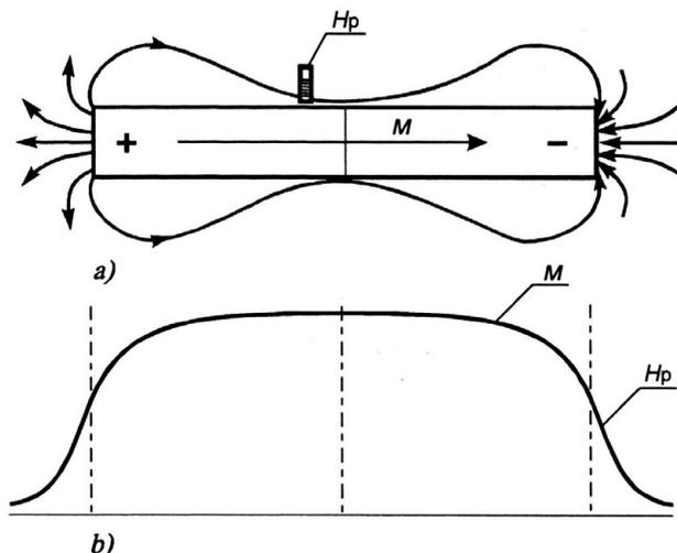
FIGURE 3. Prospective model of magnetic dipoles.
