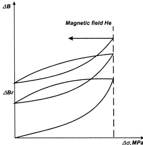
FIGURE 1. The scheme of magneto-elastic effect action:  $\Delta B_r$  – the change of residual induction;  $\sigma$  – the change of cyclic loading;  $H_e$  – the external magnetic field.
