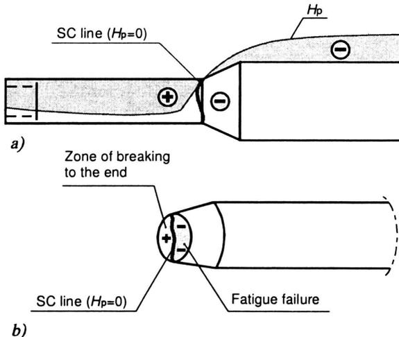
FIGURE 4. Brittle fatigue fracture of shaft.
