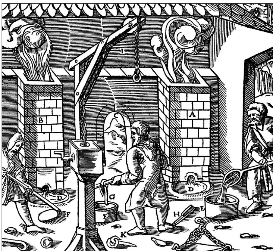
Fig. 8. Copper and lead combining furnace. After G. Agricola, 1985. fig. 253.
