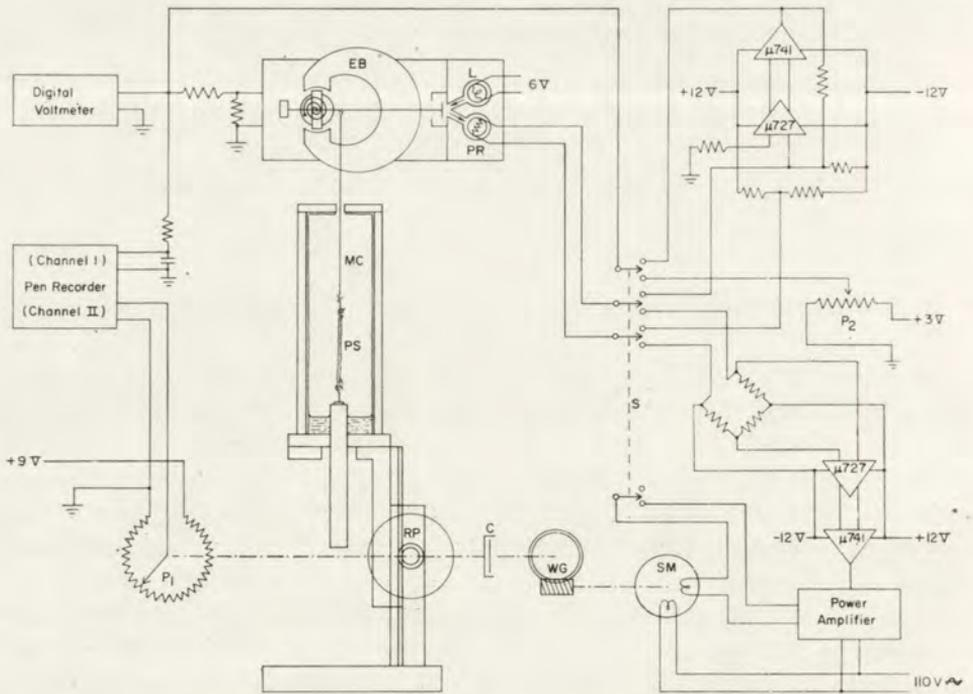
Fig. 1. Block diagram of the vertical system for measuring isometric and isotonic contraction in the hanging plasmodial strand. For explanation, see text
