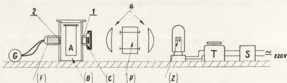
Fig. 1. Scheme of apparatus used for radiation and measurements: A — cuvette with capacity 250 ml, B — light-tight casing, F — selenium cell, G — graduated galvanometer, C — holder for interference filters and neutral net filters, Z — 1000 W projection filament bulb, T — voltage control, S — equalizer, P — thermal filter with  $H_2O$ , H — glass lenses, 1 and 2 round holes (1 containing selenium cell)
