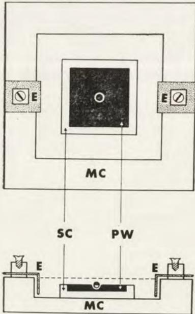
Fig. 1. Experimental chamber, vertical view, and below—horizontal cross-section. MC—main chamber; SC—small chamber; E—silver/silver chloride reversible electrodes; PW—paraffin-bee wax lining
