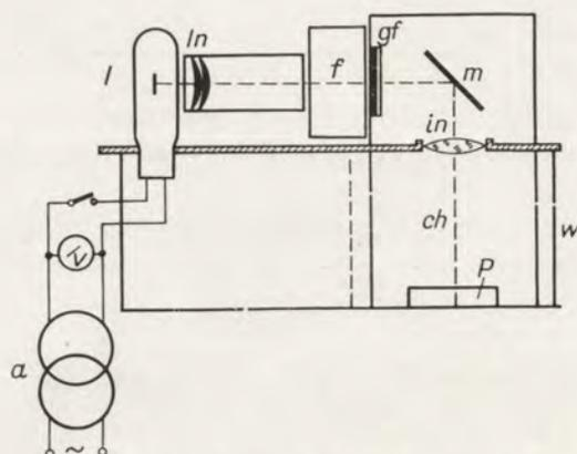
Fig. 6. Scheme of the apparatus for irradiation 1—lamp, ln—lenses, f—filter with  $\text{CuSO}_4$  solution, gf—glass filter, m—mirror, ch—chamber for illumination, P—Petri dish, v—volta-meter, a—auto-transformer, w—water jacket
