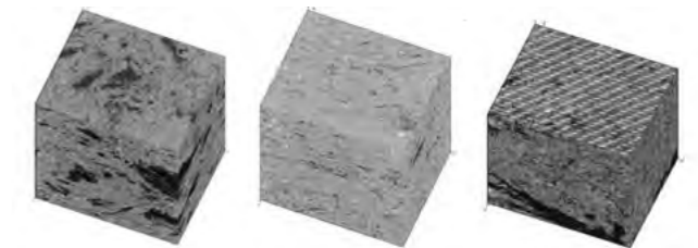
Fig. 4.2.10. Three-dimensional view of three specimens cut off the boards of different quality
