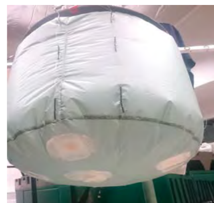
Fig. 8.8. Sensors-equipped airbag as an element of the AdBag System
