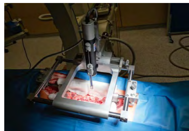
Fig. 5.5. Prototype of device for intraoperative stem cell delivery (CUL)
