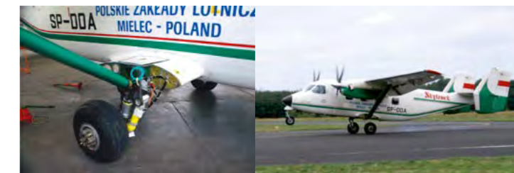
Figs. 8.6. and 8.7. Adaptive suspension landing gear mounted on M28 SKYTRUCK (left) and the aircraft, equipped with the adaptive landing gear, during landing (right)
