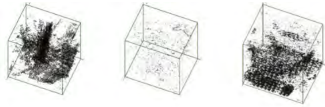
Fig. 4.2.11. Visualisation of fibres in presented specimens performed by examining the datasets resulted in micro-CT scanning
