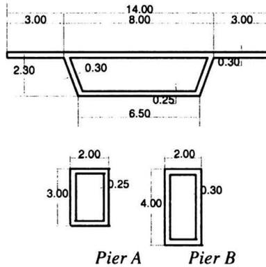
FIGURE 7. Cross sections of the deck and of the piers of the bridges depicted in Fig. 8.
