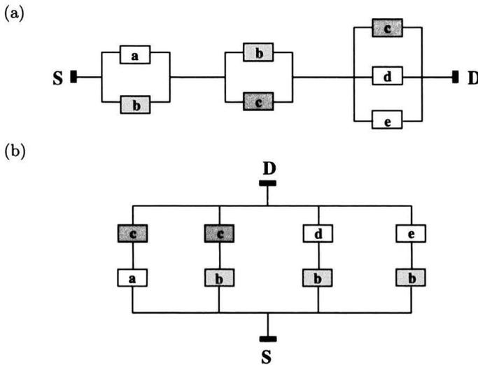
FIGURE 10. Minimal cut set (a) and minimal path set (b) representations of network CO (Fig. 8).
