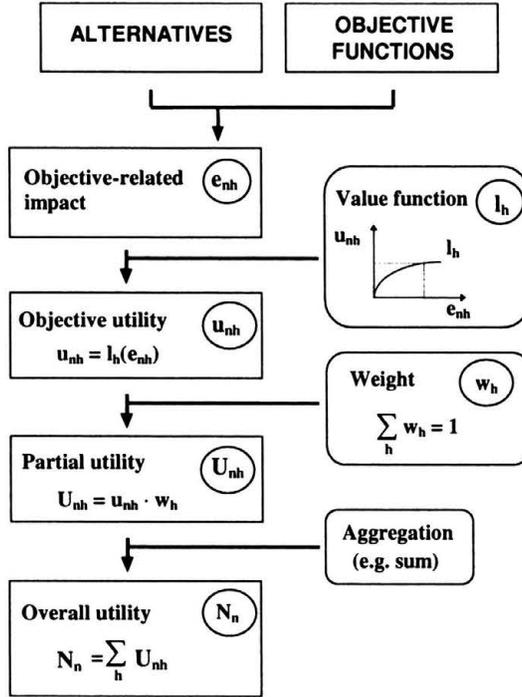
FIGURE 16. Logical diagram of Utility Value Analysis.
