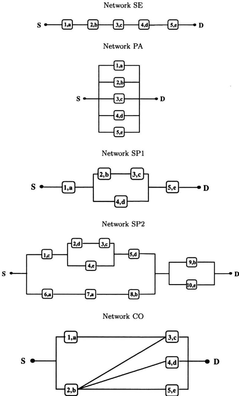
FIGURE 9. Diagrams of five example networks; locations and identification of critical elements.
