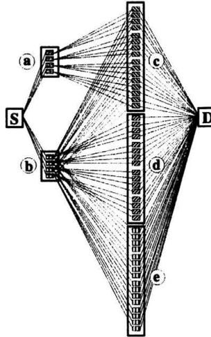
FIGURE 12. 5-node network CO transformed into an exploded graph (each node: 4 alternative conditions).
