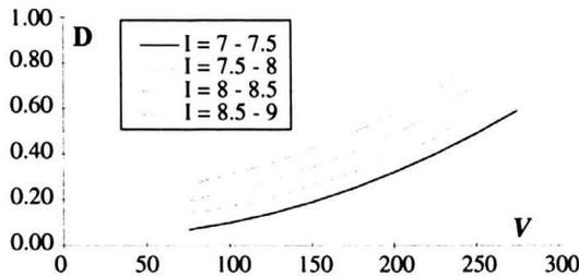
FIGURE 4. Degree of damage  $D$  vs. vulnerability index  $V$ .
