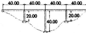
FIGURE 8. Structural diagrams of example bridges (measures in [m]).
