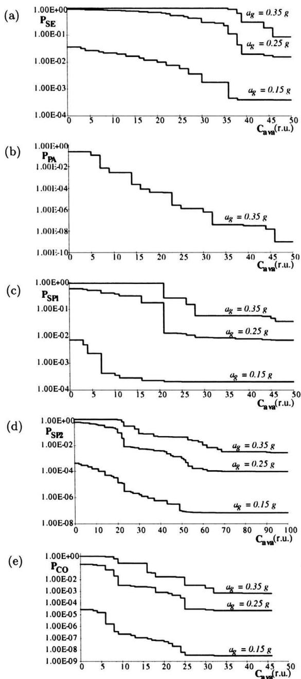
FIGURE 11. Probability of failure (loss of connectivity) versus employed resources (optimally allocated); peak ground acceleration  $a_g = 0.15 g$ ,  $0.25 g$  and  $0.35 g$ : (a) network SE; (b) network PA; (c) network SP1; (d) network SP2; (e) network CO.
