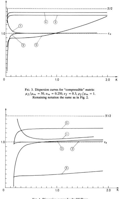
FIG. 4. Dispersion curves for "soft" fibres  $\mu_f/\mu_m = 5.0$ ,  $\nu_m = 0.333$ ,  $\nu_f = 0.3$ ,  $\rho_f/\rho_m = 1$ . Remaining notation the same as in Fig. 2 except the scale of  $\beta(1:1)$ .
