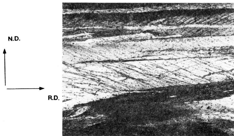
FIG. 2. Pattern of the observed copper polycrystal cold rolled to \varepsilon = 1.4 .
