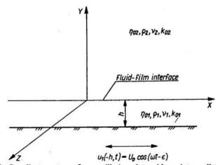
FIG. 1. Coordinate system of an oscillating plate with an intermediate film.
