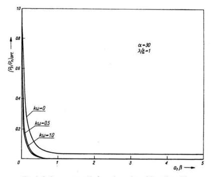
Fig. 4. Optimum power ratio for various values of  $k\omega$  and  $\alpha = 30$ .
