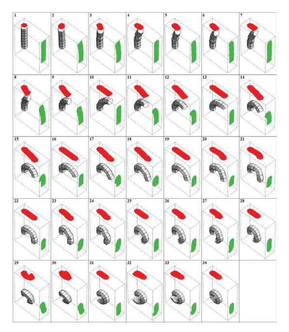
Figure 3: A possible transition from a "straight tube" to a full torus in 34 time-steps. The projections of PZ on horizontal and vertical-transverse planes are shown in red and green, respectively. The number of PZMs U = 16. The initial module (PZM<sub>0</sub>) is shown as transparent.
