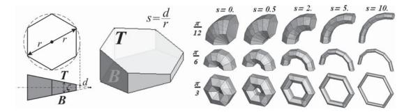
Figure 2: On the left: a visualization of PZM which is defined by parameters: r, d,  $\zeta$  and n. Since n = 6, the top (T) and bottom (B) faces are hexagons. On the right: variety of PZs constructed with the same sequence of six units with relative twists  $k_1 = k_2 = ... = k_5 = 0$  at increasing values of s and  $\zeta$  along columns from the left and rows from the top, respectively. The value of parameter r = 1, however, the images are zoomed-to-fit.
