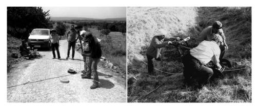
Fig. 1. Refraction seismic fieldwork (left) and GPR fieldwork (right) in Ephesos
