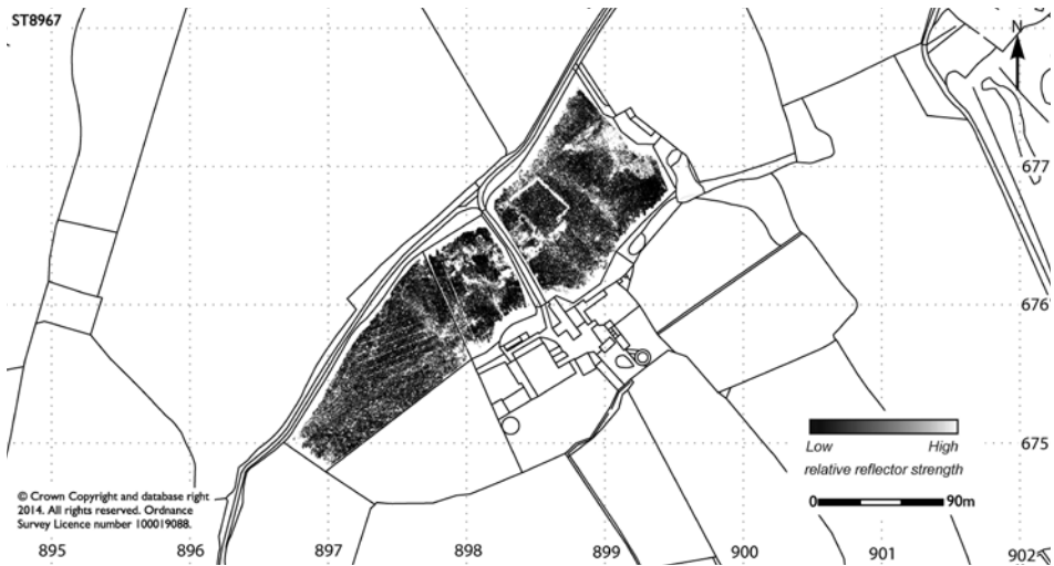
Fig. 3. Amplitude time slice between 8.4 and 9.6 ns (0.46 m to 0.53 m) from over the medieval settlement at Catridge Farm, Lacock, Wiltshire, UK. Despite the presence of water-saturated soils, the ground-coupled GPR array produced useful results to complement the analytic earthwork and magnetic surveys
