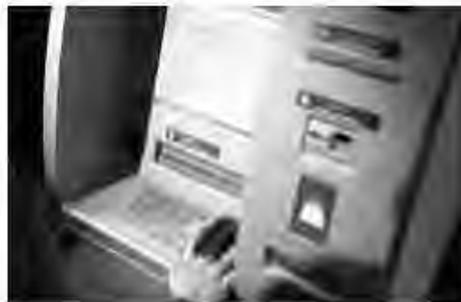
**Fig. 1.** FingerVein enabled ATM.
