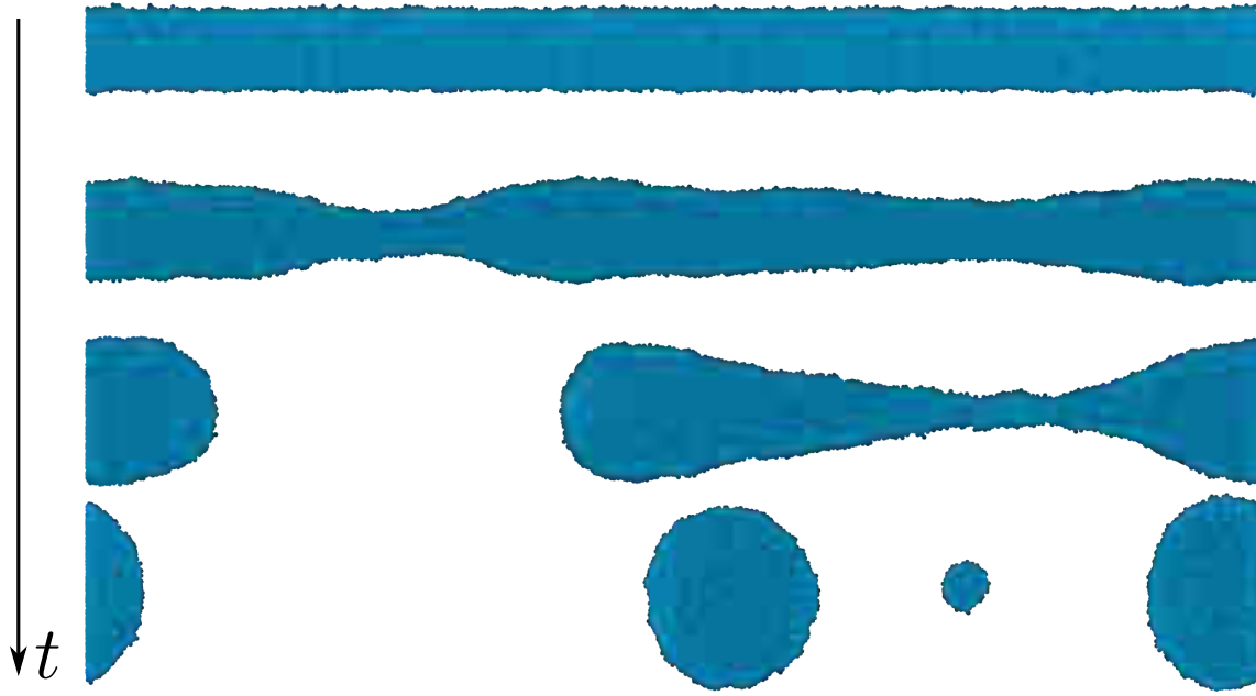
FIGURE 3.3: Characteristic snapshots from the simulations during the time evolution of the breakup from the liquid thread to individual droplets. Here, R_0 = 6 , A = -50 , L = 8\pi R_0 .
