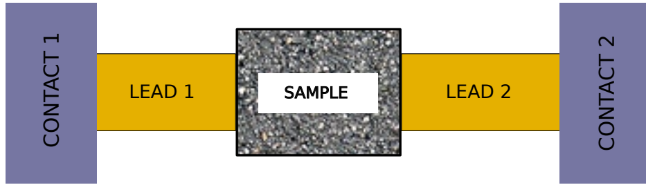
Figure 1.10: Schematic illustration of a two-terminal setup to calculate conductance through a sample. The leads here are ideal waveguides which are connected to electron reservoirs called contacts. Figure adapted from [2].
