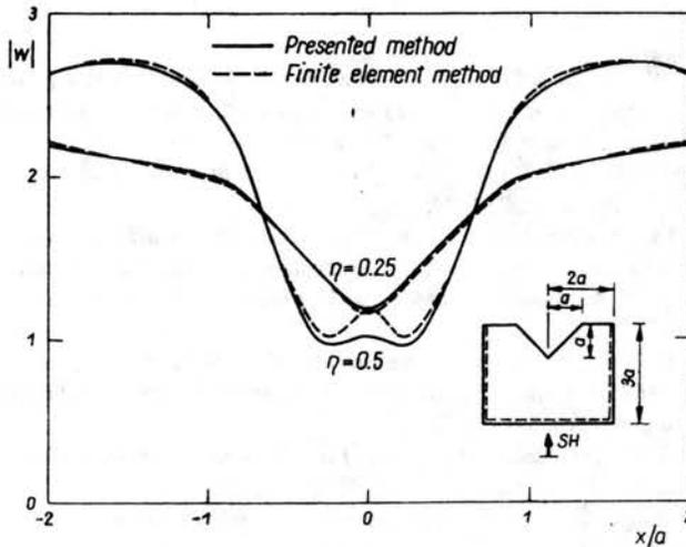
FIG. 7. Amplitudes of displacements for vertically incident  $SH$  waves  $\eta = 0.25, 0.5$ . Comparison of results with those obtained with the finite element method with efficient-active boundaries (3).
