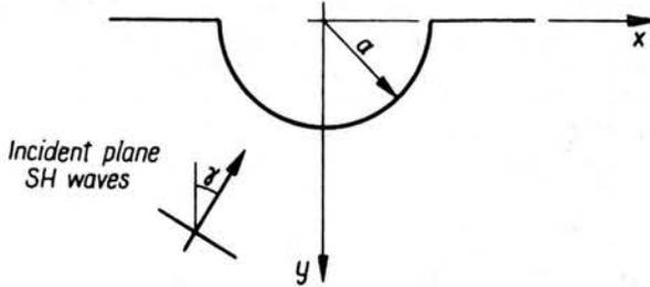
FIG. 6. Semi-circular canyon under incident plane SH waves,  $\gamma =$  angle of incidence.
