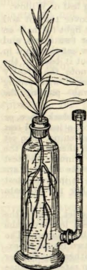
Fig. 59.—Apparatus for estimating the Absorption of Water by the Roots, and the Loss by Transpiration from the Leaves.
