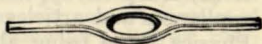
Fig. 13.—A Ward's Tube (Moist Chamber) which can be cemented to a slide.
