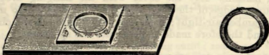
Fig. 12.—A Moist Chamber Slide; on the right, a glass ring which can be cemented to an ordinary slide, to form a moist chamber.
