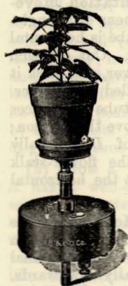
Fig. 64.—Clinostat, in vertical position as used for experiments on Phototropism.
