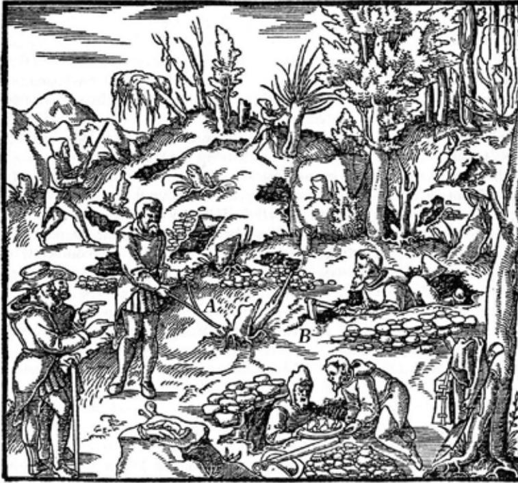
Fig. 1. Ore prospecting by Agricola (1556). A – dowsing rod, B – prospecting trench
