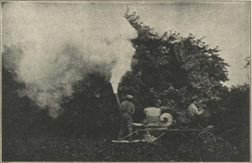
FIG. 192.—Dusting apple trees with an engine-driven orchard duster. (From Niagara Sprayer Co.)
