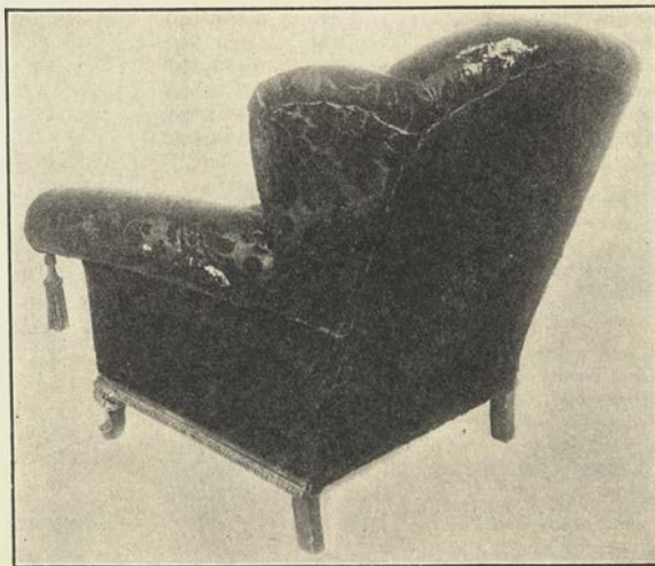
FIG. 17.—Overstuffed winged chair damaged by clothes moths. The bare spots were caused by the moths eating beneath the cover, resulting in the falling out of the mohair pile. (From Back and Cotton , U.S.D.A.)
