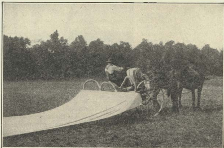
FIG. 306.—Four-row traction duster equipped with "trailer" to hold the fumes from nicotine dust. (From U.S.D.A., Farmers' Bul. 1499. )
