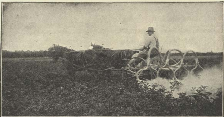
FIG. 190.—Dusting potatoes with a two-horse field-crop traction duster, with discharge pipes arranged to cover four rows. (From Niagara Sprayer Co.)
