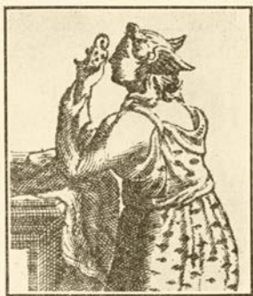
FIG. 54.—To SHOW HOW THE LEEUWENHOEK MICROSCOPE WAS HELD. (Petri.)
