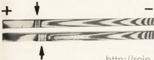
Fig. 5. Sedimentation of initial (above) and phage-treated (below) Vi-polysaccharide (2 mg./ml.) in (a) 0.05 M-HCl-veronal buffer, pH 7.8; and (b), 0.1 M-acetate buffer, pH 4.7, in analytical ultracentrifuge Spinco model E. Photographs were taken after 80 min. centrifugation at 56 100 rev./min. at 18°. Centrifugation from left to right.
