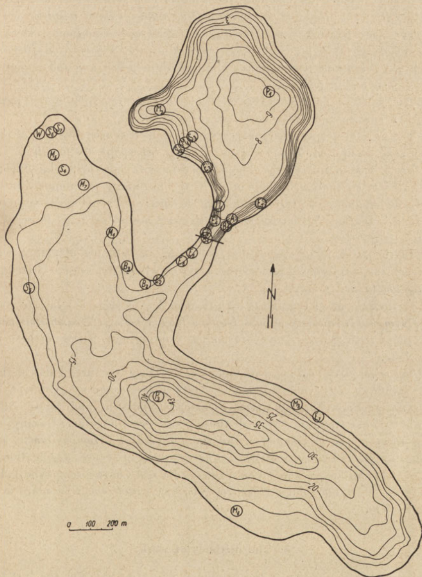
Map 1. Harsz Lake. Bathymetric Plan. Dots indicate sand-banks. Inside the circles-symbols denoting habitats. The situation of the lake: 21^{\circ}46',25'' E lat., 54^{\circ}9' N long. It is elevated 118 m. above M. S. L. The area of the lake is about 228, 1 ha
