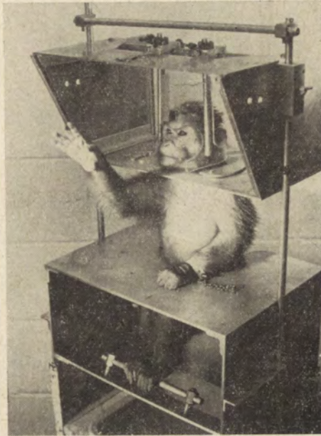
Fig. 1. Monkey in the restraining chair. Note: chain attached to monkey's right wrist and the plastic head restrainers
