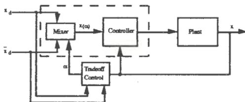
Figure 3: A scheme for the control of uncertain plant.
